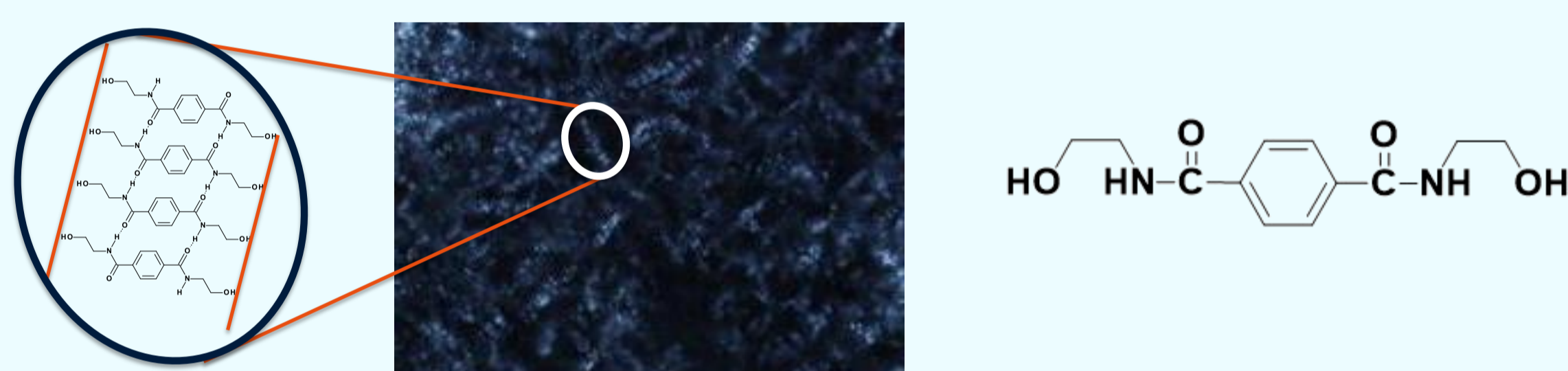
Figure 2: left: Crystal structure of self assembled nucleating agent in PLA right: The chemical structure of terephthalic based nucleation agent [N1,N4-bis(2-hydroxyethyl) terephthalamide]
